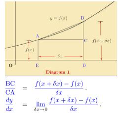
The limit, dy/dx, is called the *derivative* of the function f(x). Its value is the *gradient of the tangent* to the curve at the point A(x, y).
